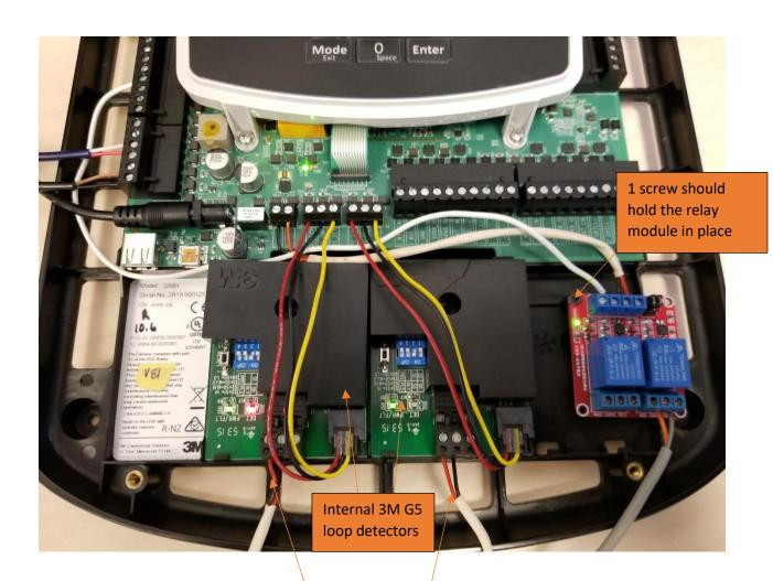
Connections to the internal detections from the ground loop for both menu and window service points
